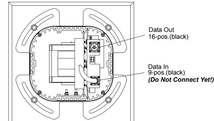
**CAUTION:** Do not connect black 9-position elec. input connector until wiring is complete and verified (See step 27).
