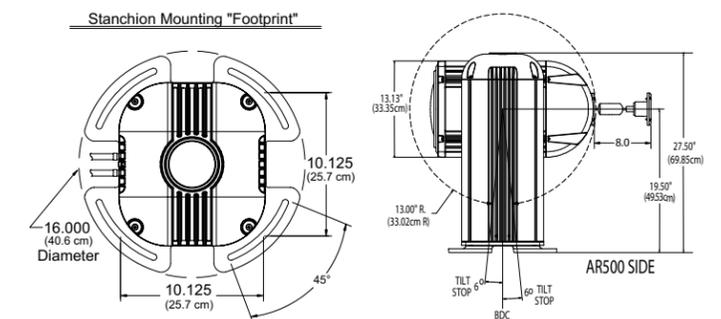
The luminaire head tube is installed through a hole in the side of the stanchion. The luminaire head rotates 348 degrees from stop to stop. Allow at least eight inches (203mm) clearance behind the luminaire head for lamp removal and replacement.
