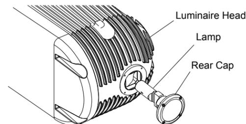
18. Install lamp in lamp socket. Do not touch the quartz bulb with bare fingers. If touched, clean quartz bulb with alcohol.
