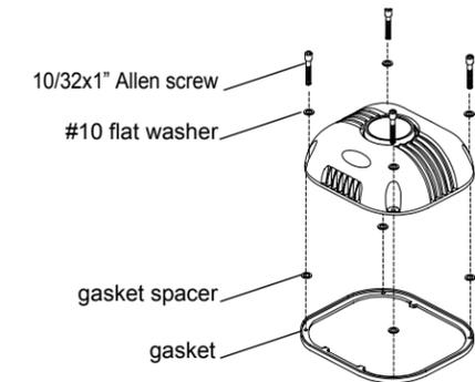
**Note:** Ensure #10 washers and gasket spacers are installed as pictured above.
