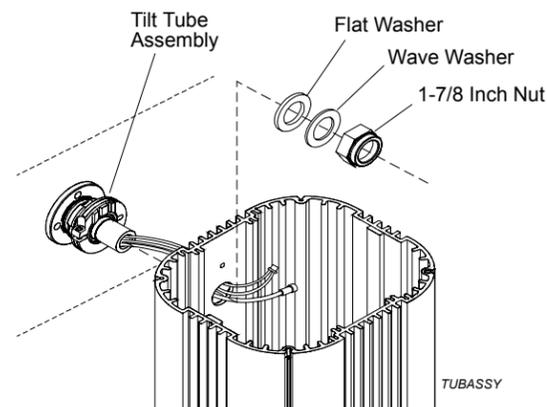
6. At head assembly, remove nut, spring washer, and flat washer from head enclosure tilt tube and from cables. **Ensure black o-ring stays in tilt tube groove.**
